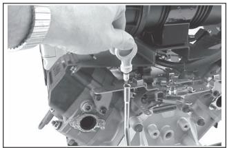
Figure 6. Checking Oil Level.
